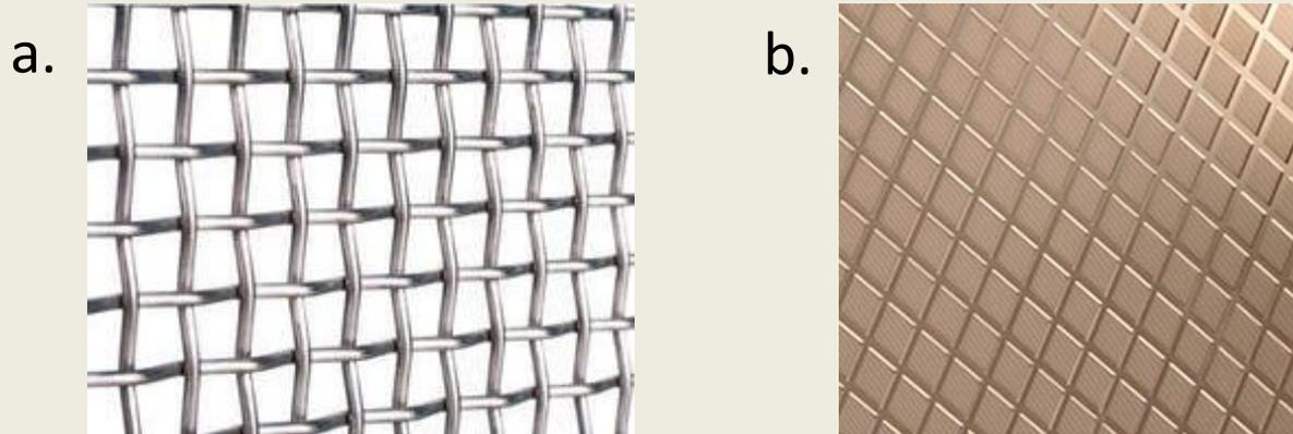
Photomicrographs of (a) Woven-wire screen and (b) micromesh screen
